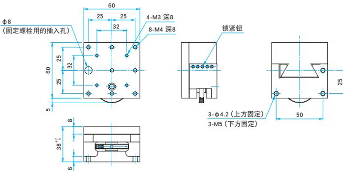
**TASB-653-M6/653UU** 内六角螺栓 M6×12...3个, 1.5mm六角扳手...1个, 5mm六角扳手...1个(M6) 内六角螺栓 1/4-20UNC×1/2...3个, 1.5mm六角扳手...1个, 3/16inch六角扳手...1个(UU) 锁紧钮用扳手尺寸1.5mm, 六角扳手サイズ5mm(M6) 锁紧钮用扳手尺寸1.5mm, 3/16inch取付ネジ締付用(UU)
