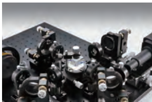
A movable mirror for changing the optical path difference
