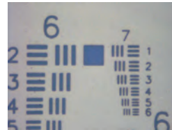
ZRCL-1.5 Observation Field of View About 0.37x0.3mm
