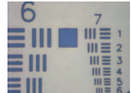
ZRCL-2 Observation Field of View About 0.28x0.22mm
